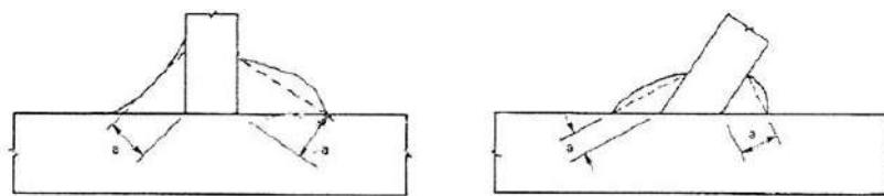
Figure 4.3: Throat thickness of a fillet weld
