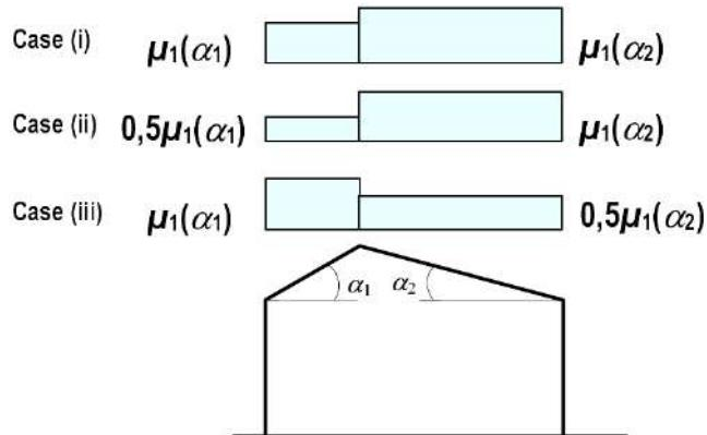
The snow load shape coefficients that should be used for roofs abutting to taller construction works are given in the following expressions:
