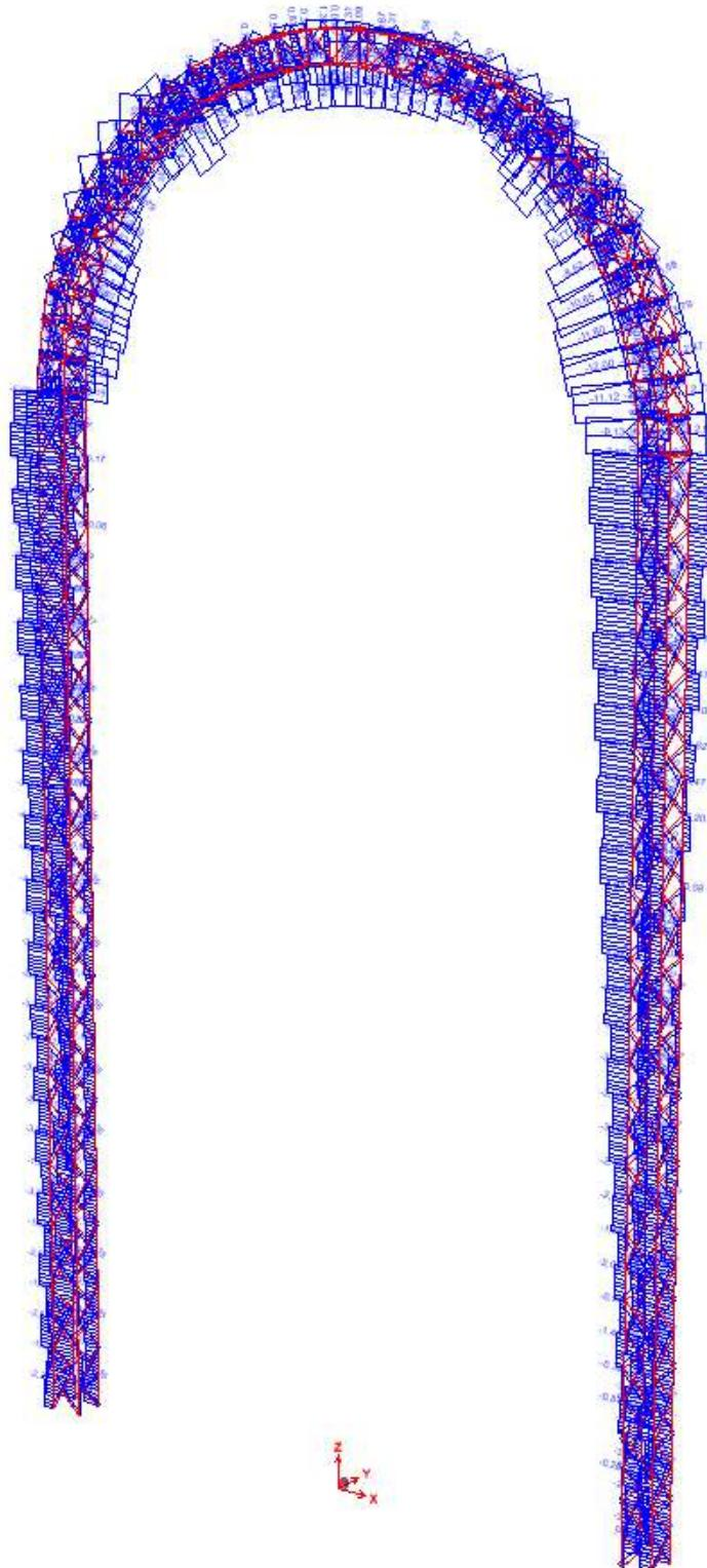
*f.e.m model of antennas - axial force (envelope values kN)*
