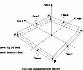
Four-node Quadrilateral Shell Element
