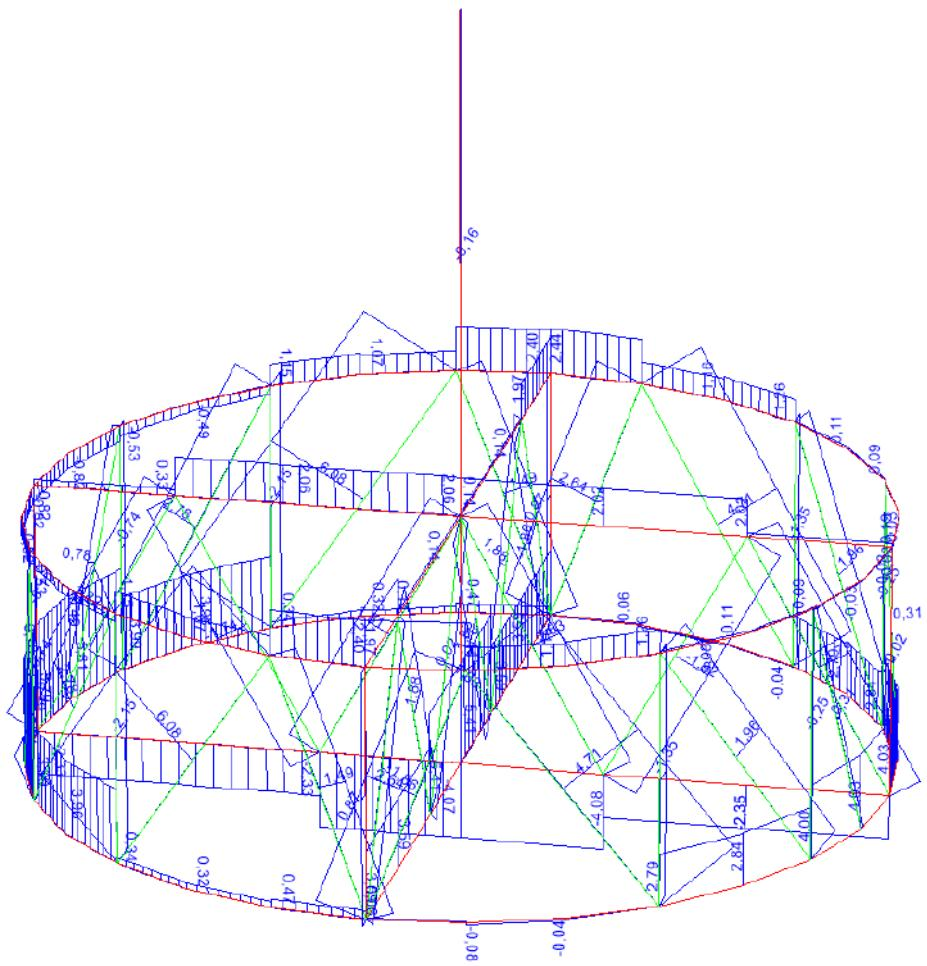
f.e.m model of upper ring - axial force (envelope values kN)
