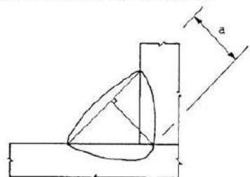
Figure 4.4: Throat thickness of a deep penetration fillet weld
