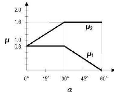
The values apply when snow is not prevented from sliding off the roof. Where snow fences or other obstructions exist or where the lower edge of the roof is terminated with a parapet, then the snow load shape coefficient should not be reduced below 0,8.
